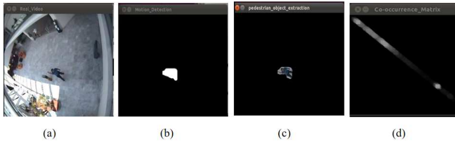
Fig.1. (a) Frame 154, (b) Moving Object Detection, (c) Moving Object Extraction, (d) Co-occurrence Matrix computed within moving object region (c).
